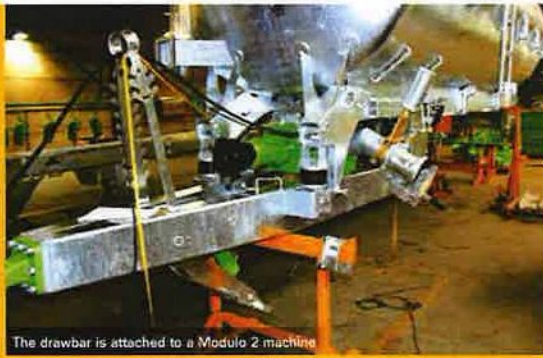
The drawbar is attached to a Modulo 2 machine
